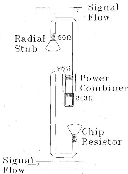
Fig. 2. Detail of a single tap-cell.
