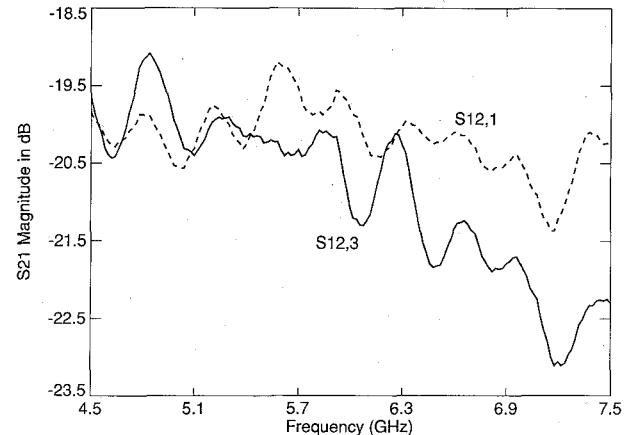
Fig. 3. Comparison of  $S_{21}$ -frequency response of eight port when fed from ports one and three.
