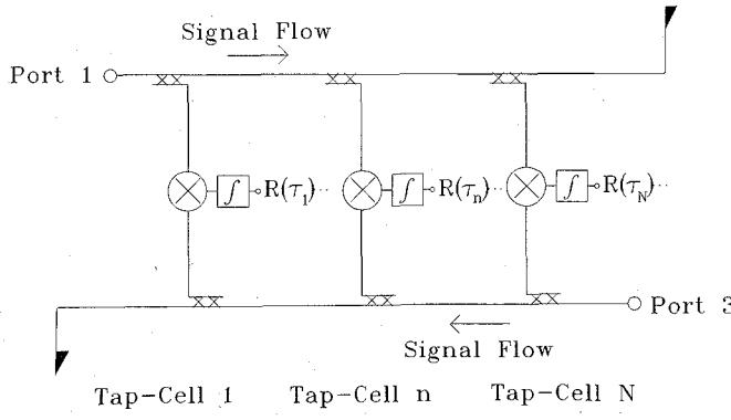
Fig. 1. Schematic of the parallel delay line circuit.
